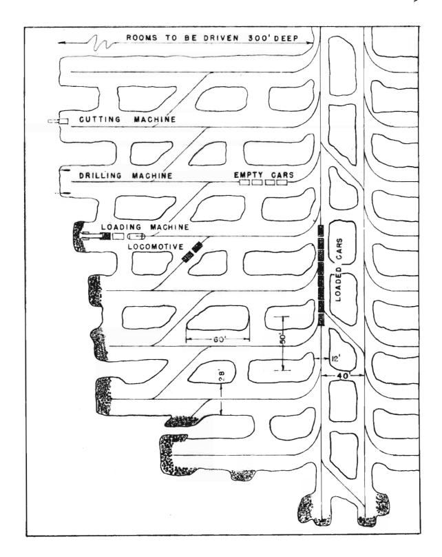
Fig. | Advancing panel system with mobile loader and one battery locomotive.
