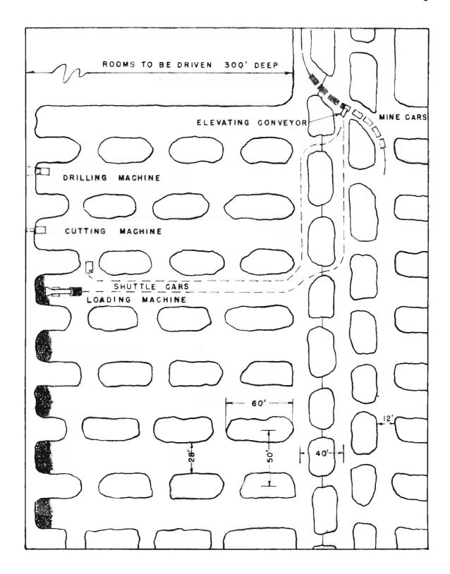
Fig.2 Advancing panel system with mobile loader and two cable-reel shuttle cars.
